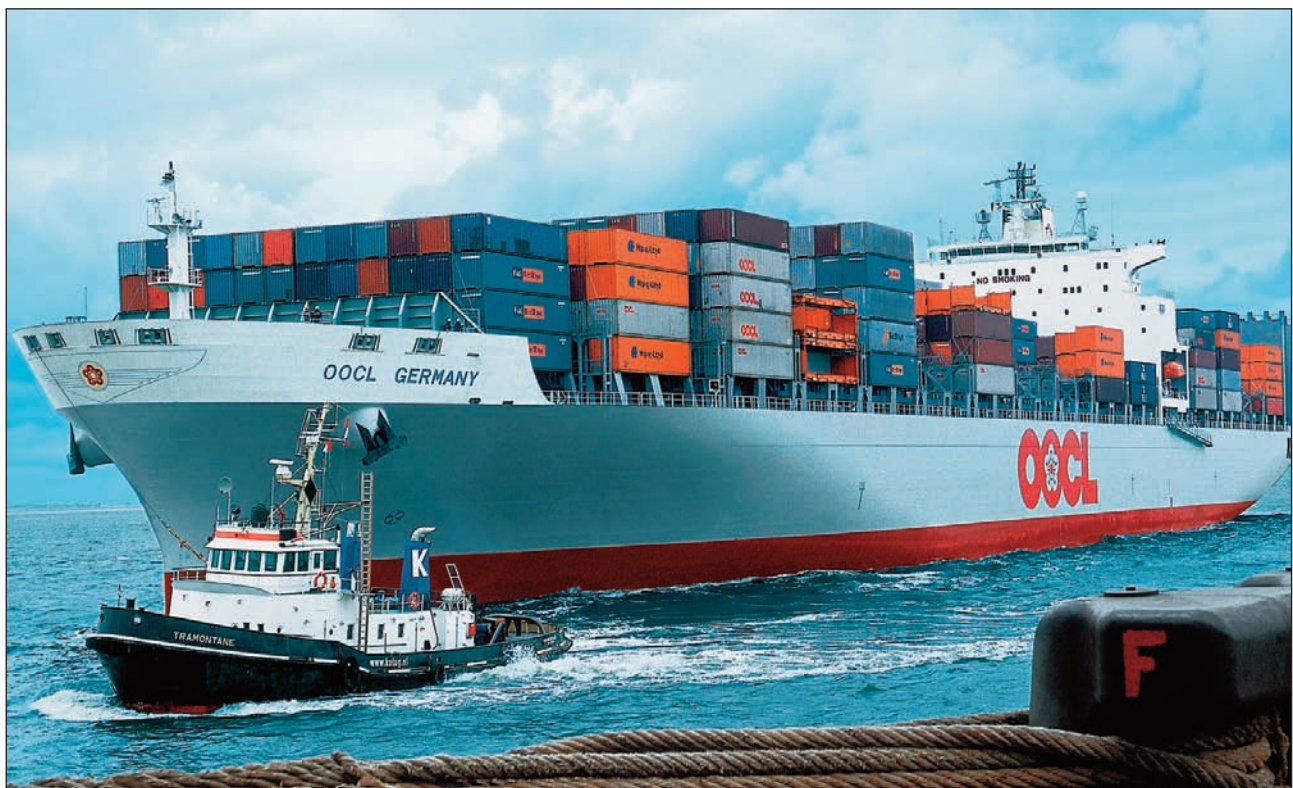
The M/V "OOCL Germany" (above) a Panamax class ship. It is 277 m long, 40 m wide and can carry 67 500 tons in a 14 m draught. Maximum speed is 26.1 knots. Photo provided by E.R. Schifffahrt
